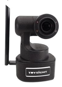
The NEW Magnibot from Trysight is a wireless battery-powered robotic distance camera that is perfect for the classroom. Connect the Magnibot to an iPad, Chromebook or any device with a web browser and control the camera wirelessly from that device! There are no cords to hassle with and setup is a breeze!
