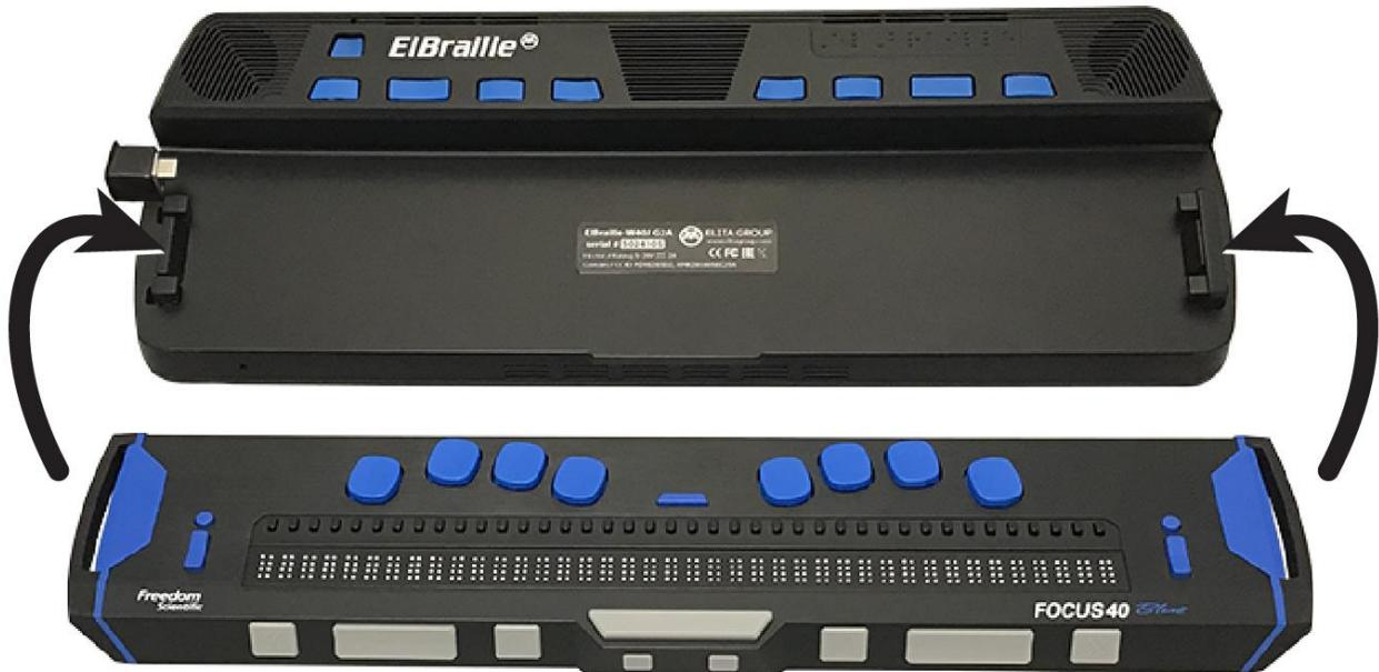
3. Push the locking lever to lock the display in place and establish the USB connection.
