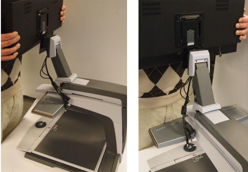
C) Connect the VGA, power and USB cable to the monitor and to the ClearView+
